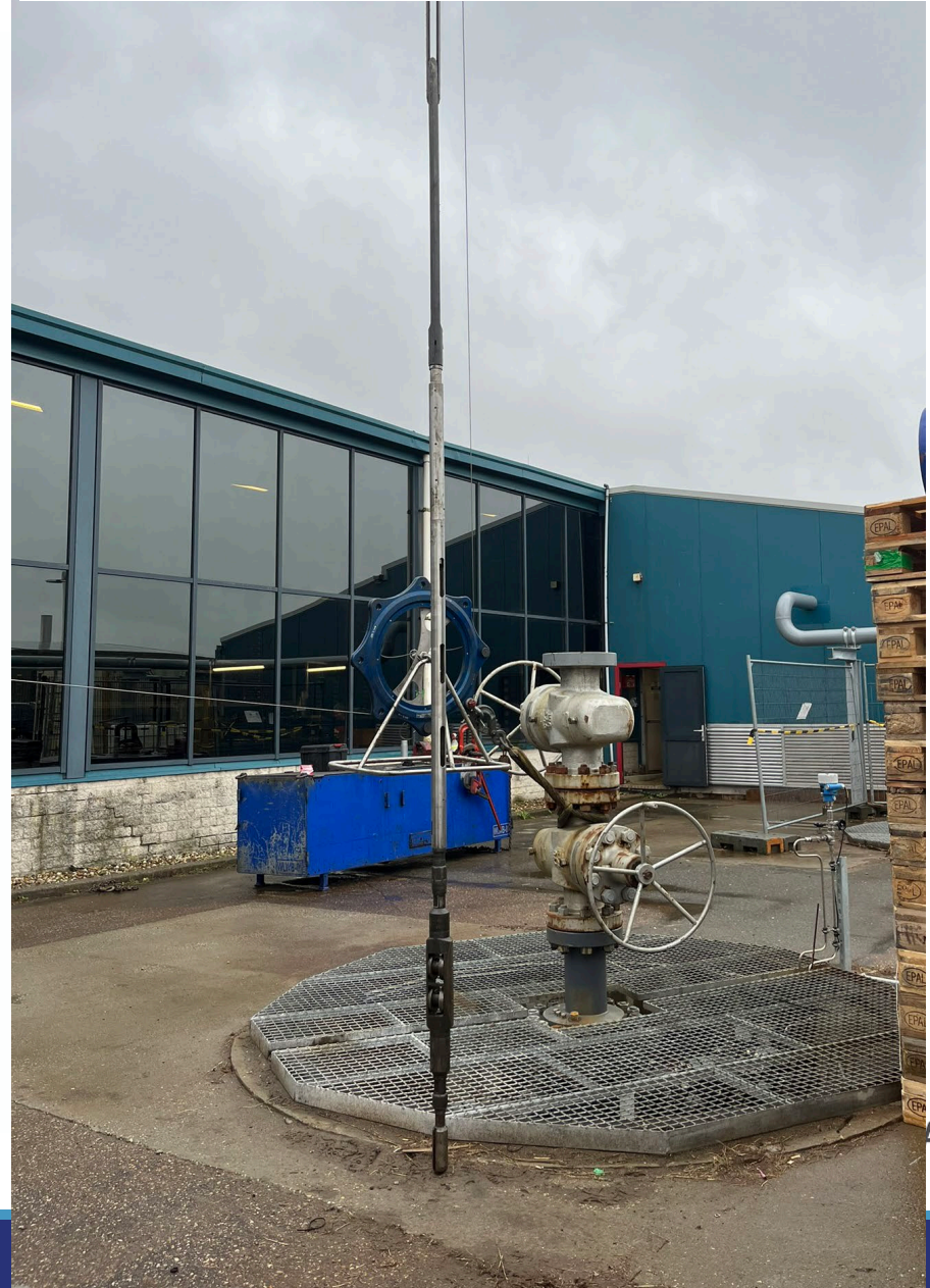
Toolstring: slickline with jar, PT memore gauge, bull nose.
